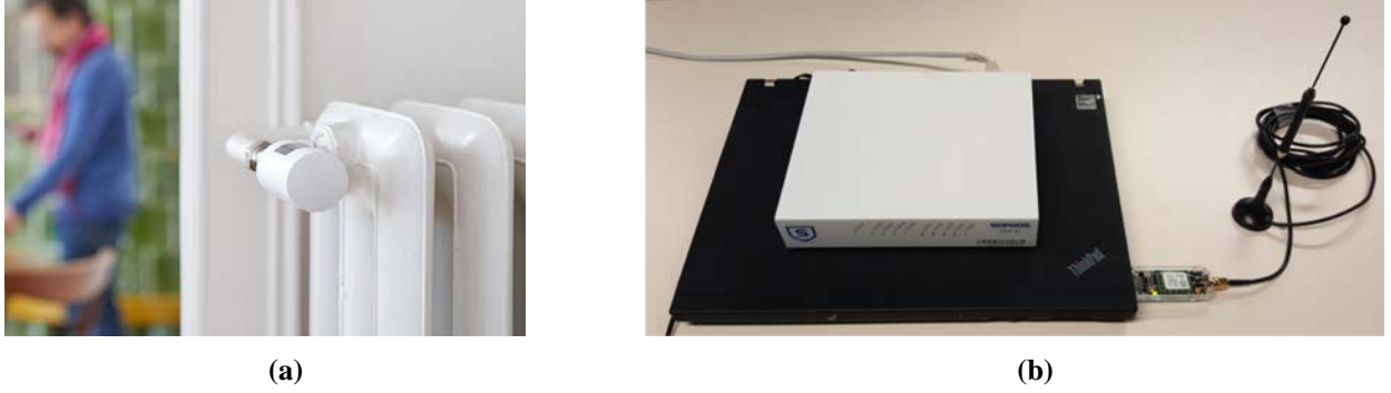
Fig. 2. (a) SmartDrive-MX STV from HORA; (b) logging PC with EnOcean dongle and RED.
