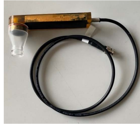
Fig. 3. INRIM transducer comprising an SU103 S/N 101, Sonic Concepts transducer with stand-off cone, which was filled with deionized, degassed water, and fitted with a Mylar acoustic window for measurements.
