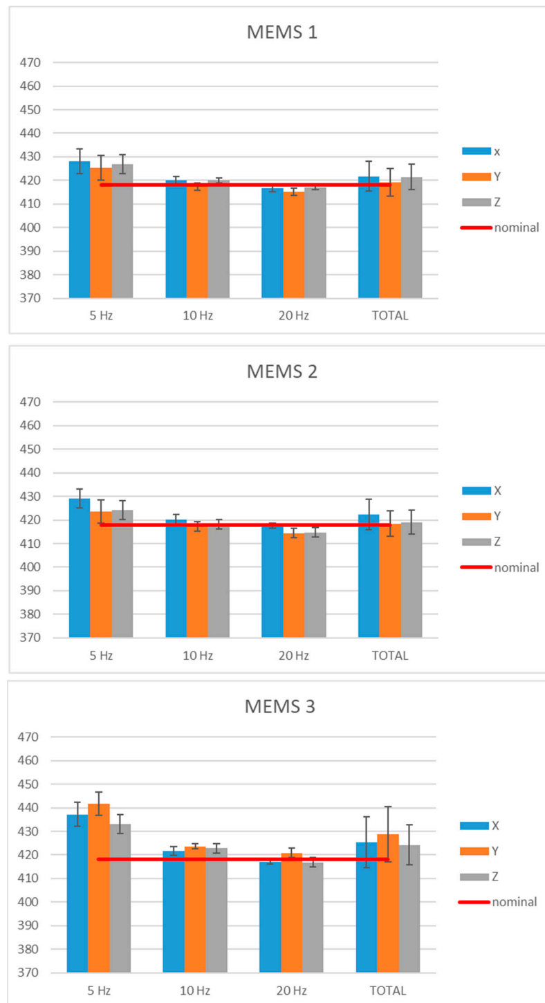
Figure 8. Sensitivities along the X-axis, Y-axis, and Z-axis of the digital MEMS subjected to linear motions.
