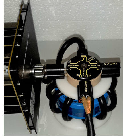
Fig. 5. Current node with built-in current choke for operation up to 20 A with an example of the current shunt insertion. In particular, the gold dual binding post banana jacks have center to center spacing of about 10 mm and are encapsulated into an epoxy compound. A short twisted pair cable with banana plug termination is used to connect the current measurement input of single and three-phase standard wattmeters and watthour/varhour meters under calibration.
