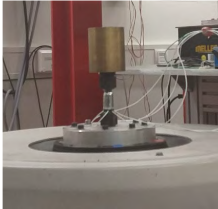
Figure 45 self-manufactured strain gauge on the electrodynamic shaker
