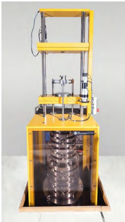
Figure 3 Deadweight 20 kN force standard machine (FSM) at PTB Braunschweig (left), typical mounting of the transducer for tension mode (upper right) and typical mounting of the transducer for compression mode (lower right)
