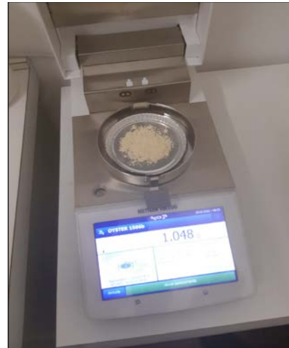
Figure 3: The desiccators (left) and the thermo-balance (right) used to measure the moisture mass fraction.
