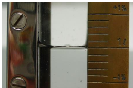
Figure 1. Standard test measure meniscus
