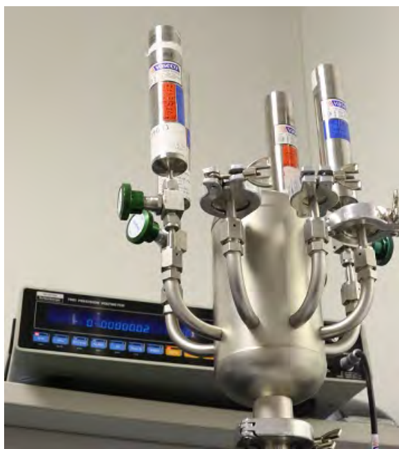
Figure E1.7.1: Reference leaks externally mounted on a leak detector (photograph courtesy of Vaseco Ltd.)
