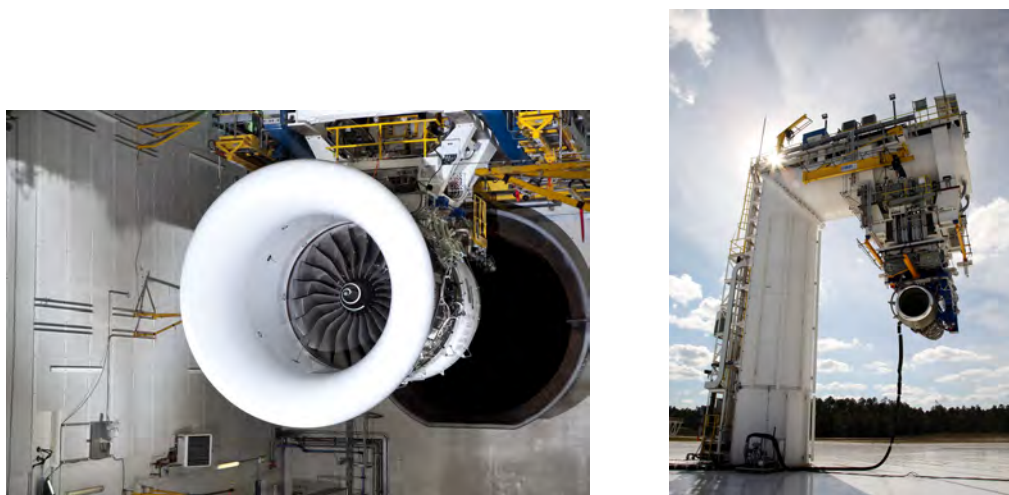
Figure E6.1.1: Test facilities for indoor (left) and outdoor (right) data acquisition
