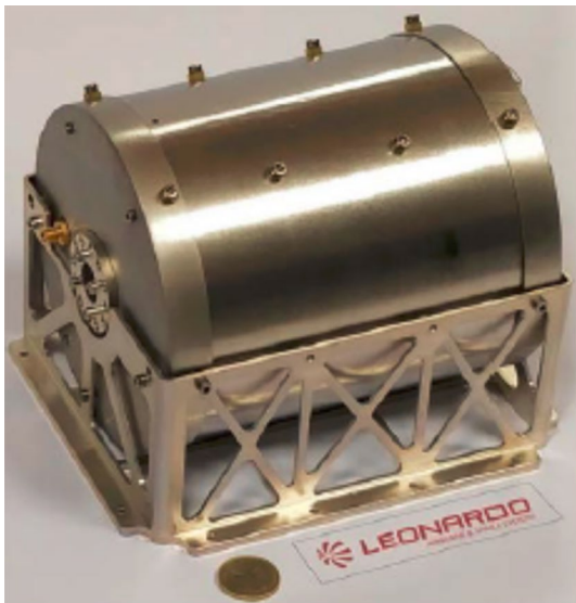
Fig. 9 POP physics package implemented by Leonardo and tested at INRIM (courtesy of Leonardo SpA). The package includes the cavity-cell arrangement, magnetic and thermal shields, whereas the laser, its stabilization, and the AOM are part of another module. As a benchmark, a one Euro coin has been added (diameter 23.25 mm)
