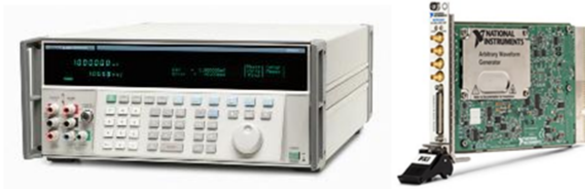
Figure 1.11: Power source - Fluke 5720A (Left) & AWG - NI PXI-5421 (Right).
