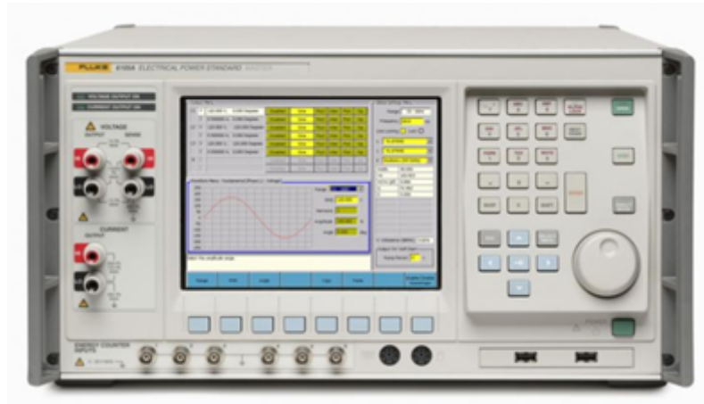
Figure 1.10: Power source - Fluke 6100A.
