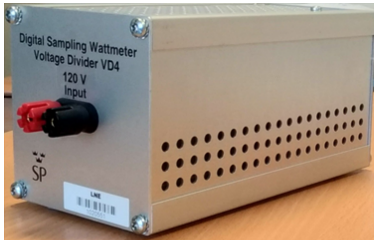
Figure 1.15: RISE Resistive Voltage Divider (RVD).
