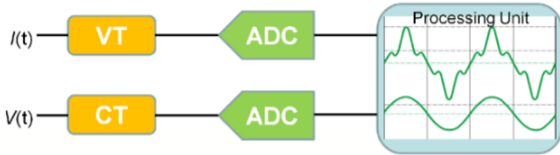
Figure 1.33: Basic structure of synchronized digitizers in a digital sampling wattmeter.
