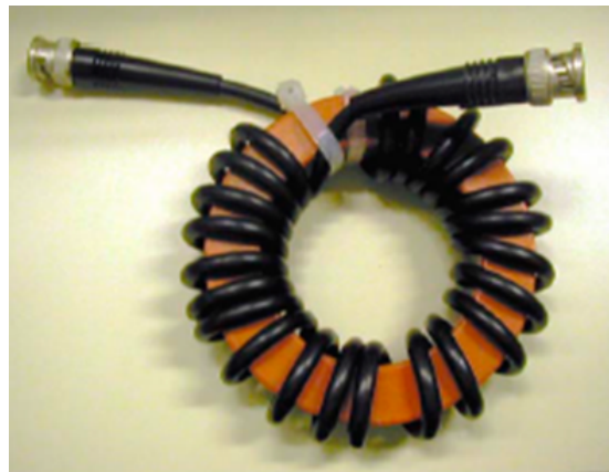
Figure 1.9: Current equalizer (Choke).
