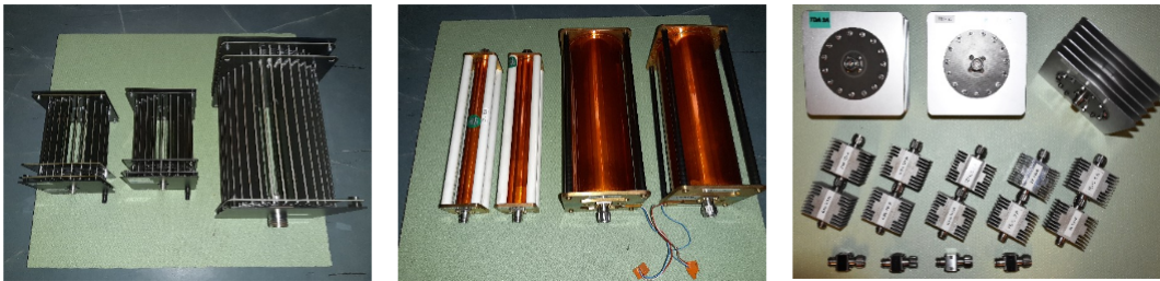
Figure 1.37: Coaxial shunts: (Left) Cage design (manufactured by Fluke), (Middle) Coaxial foil structure (manufactured by BEV), (Right) Coaxial disk design (manufactured by INRIM).
