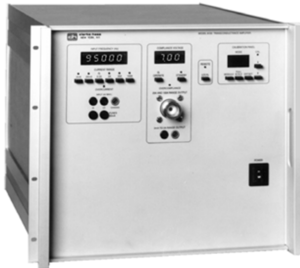
Figure 1.13: Transconductance amplifier - Clarke Hess 8100.
