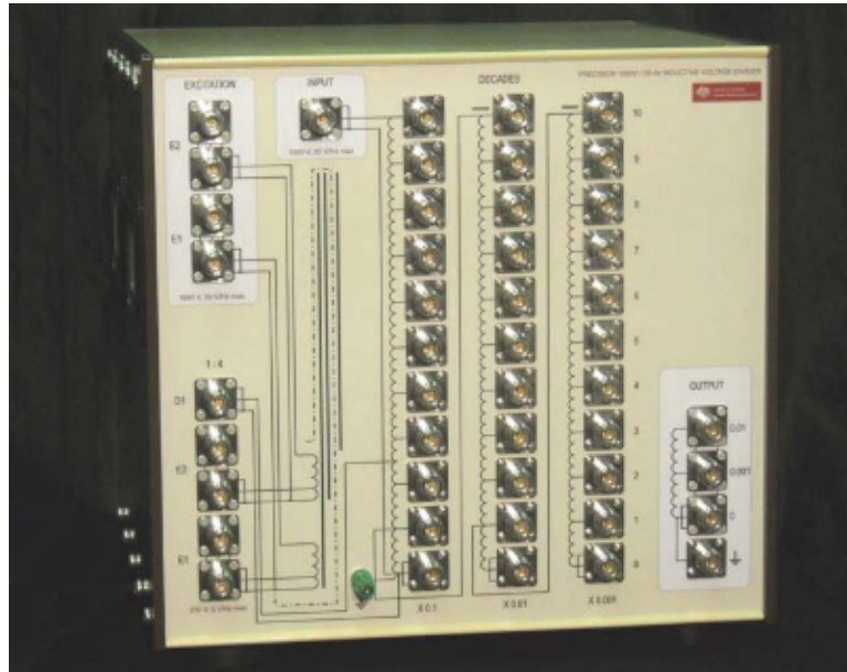
Figure 1.14: NMIA Inductive Voltage Divider (IVD) [8]
