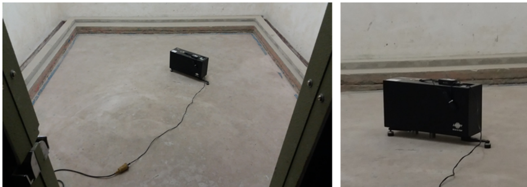
Figure 3: Normalized laboratory of impact sound insulation at INRIM: the reference base floor and the standard tapping machine.
