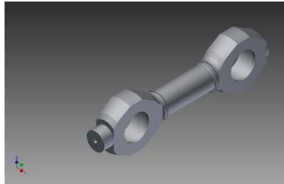
Fig. 1 Structure of the uniaxial force transducer (UFT)
